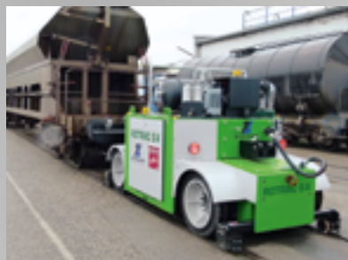
ROTRAC E4 Shunting capacity up to 500 t
