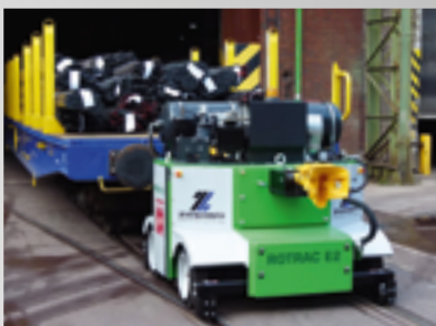
ROTRAC E2 Shunting capacity up to 250 t
