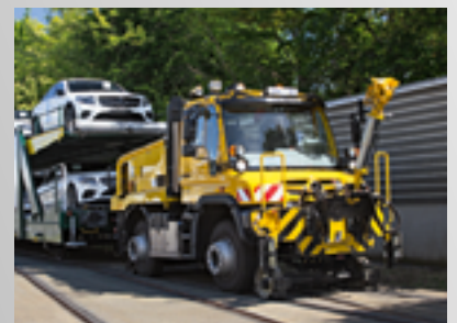
UNIMOG Shunting capacity up to 1000 t
