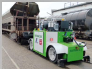
ROTRAC E4 Shunting capacity up to 500 t
