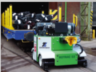
ROTRAC E2 Shunting capacity up to 250 t
