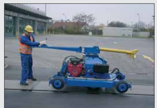
On-tracking on level-plane tracks
